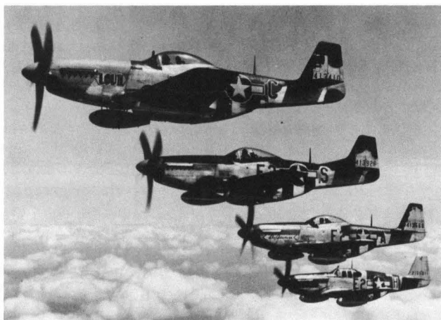
A formation of P-51 Mustangs from the 375th Fighter Group. The lowest P-51 is a B-model, while the rest are D-models.
