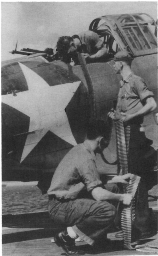
A Dauntless having its two rear .30 caliber machine guns rearmed with 1,000 rounds each. Courtesy of the U.S. Navy
