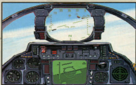
The HUD in Combat mode. Note the vertical Target Range and Closure Scales at either side.
