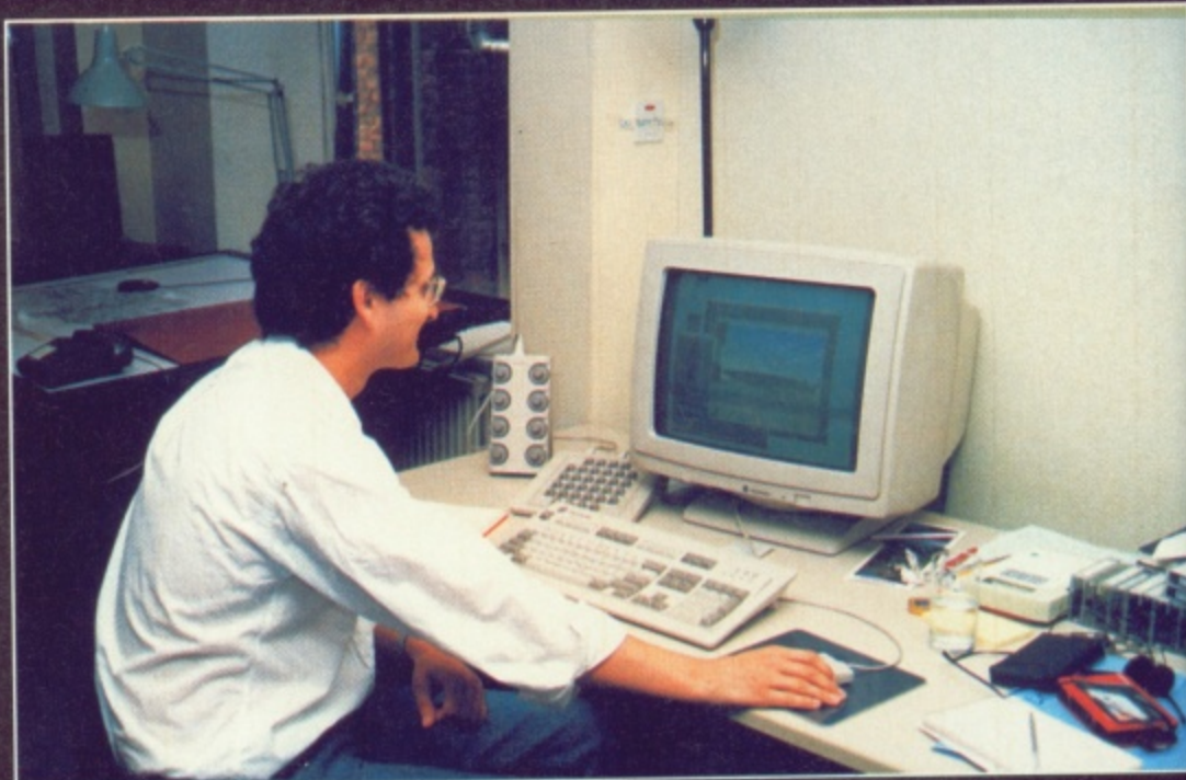
(Below) The software allows the city to be viewed from just about any angle. Jan inputs the camera's flightpath around the buildings by just setting a few key points along its route. The program then uses a process called 'splining' to calculate a smooth path between these points. Jan can watch the current flightpath in wireframe and make any adjustments necessary.
