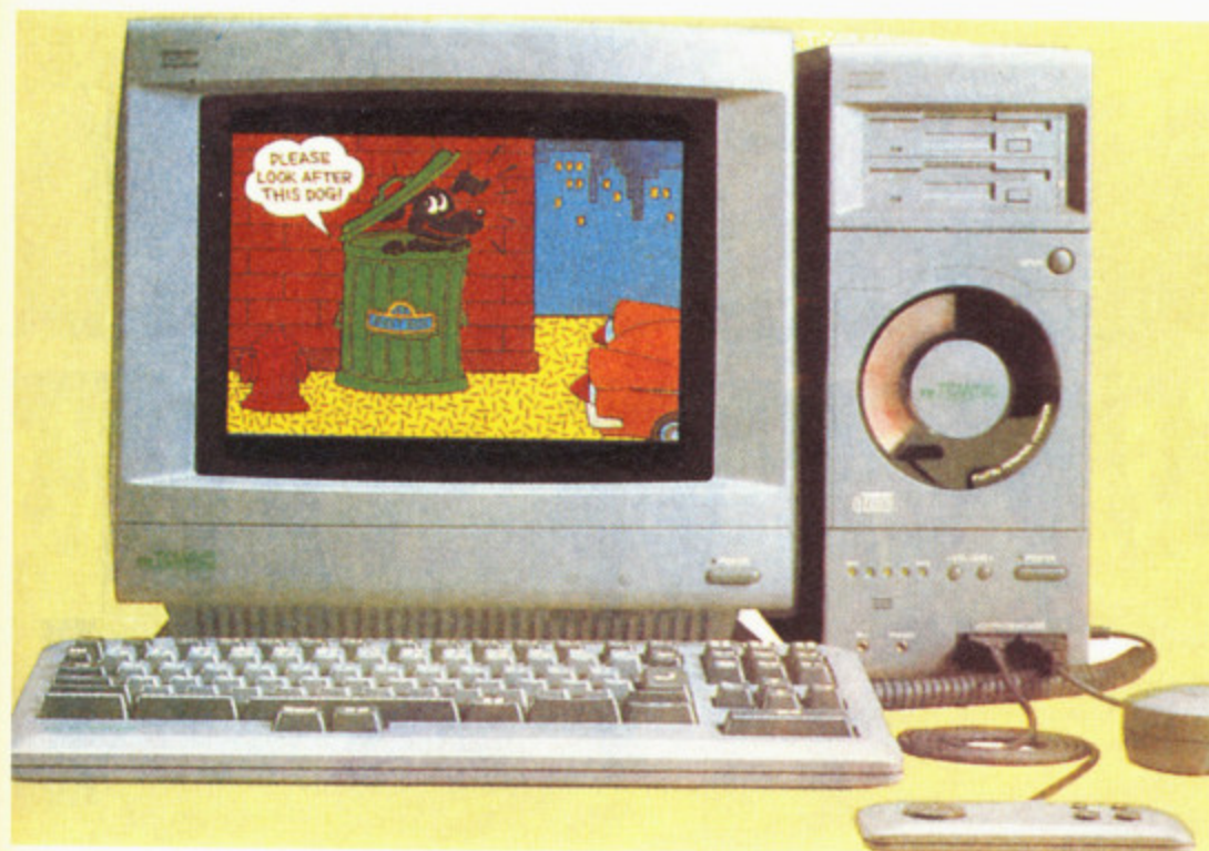
The Fujitsu FM Towns' compact design is not just designer whimsy: the machine was developed with Japanese sitting rooms in mind, and when you've seen one of those you'll understand the need for a compact machine. Although the Towns has only sold in comparatively small numbers, it enjoys a very high prestige amongst Japanese gamers.
