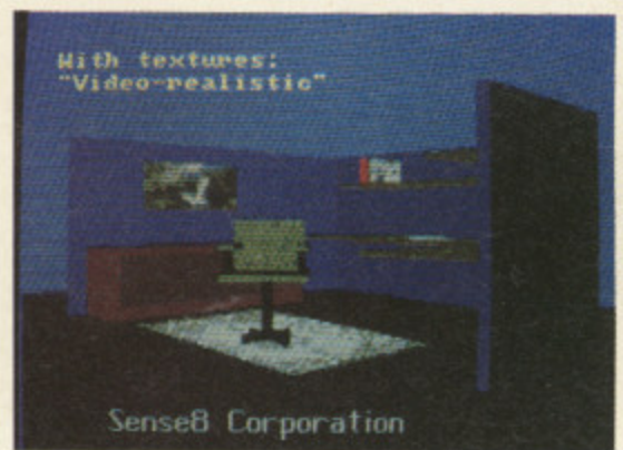
Using DVI hardware, the Intel/Sense8 DVI-VR project has produced a system for around £9000 that not only performs real-time rendering, but real-time texturing as well. Images can be stored as textures and wrapped or layered onto objects - zoom in and look at that painting and you'll be amazed by the detail
