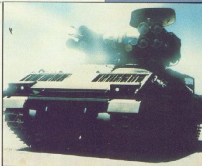
ADATS carries eight laser-beam-riding missiles that travel more than three times the speed of sound.
