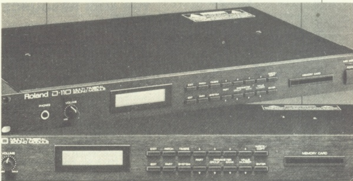
Roland's D-110 - using samples as waveforms to create some stunning sounds.
